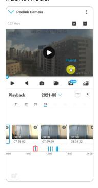
4. Tap **show alarm** icon on the bottom to show the alarm recordings only. For cameras with human/vehicle detection, you can select motion recording type of **Person,Vehicle** or **Others** to replay.
