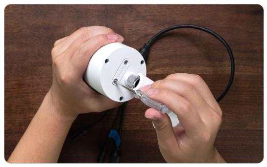
2. Find the micro SD card slot and please use something sharp such as the reset pin or a paperclip or your fingernail to push the SD card to make it pop out.
