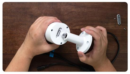
2. Insert the micro SD card like the way in the picture below, please use your fingernail (or use the provided reset needle) to push the micro SD card in until you it is locked, and you will hear a click sound and the micro SD card will not pop out if it is inserted in properly.
