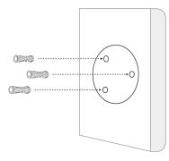
Step 4. Secure the camera in place by tightening the screws.
