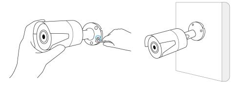
Step 5. If you want to adjust the angle of this camera, you can loosen the screw toward the direction of Unlock symbol.
