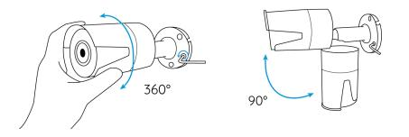
Step 2. Tighten the screw toward the direction of the Lock symbol after you adjust the camera to a suitable angle.
