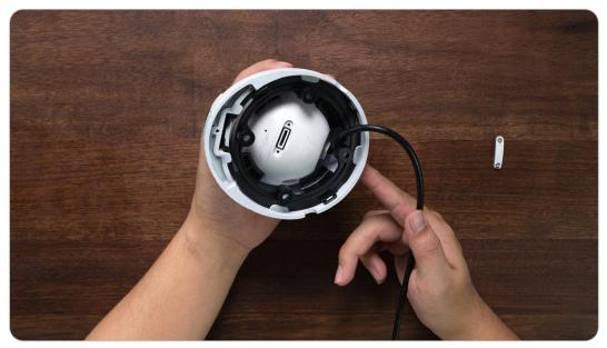
Step 2. Insert the micro SD card just like the way in the picture below, please use your fingernail (or use the provided reset needle) to push the micro SD card in until it is locked, and you will hear a click sound and the micro SD card will not pop out if it is inserted in properly.
