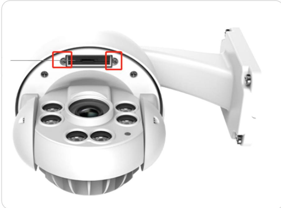
Step 2. Insert the micro SD card just like the way in the picture below, please use your fingernail (or use the provided reset needle) to push the micro SD card in until it is locked, and you will hear a click sound and the micro SD card will not pop out if it is inserted in properly.
