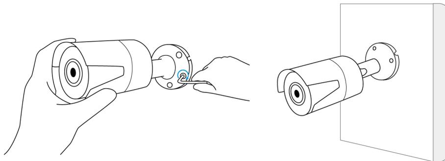
Step 5. If you want to adjust the angle of this camera, you can loosen the screw toward the direction of Unlock symbol.
