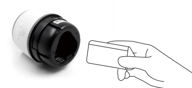
2. Find the micro SD card slot and please use something sharp such as the reset pin or a paperclip or your fingernail to push the SD card to make it pop out.
