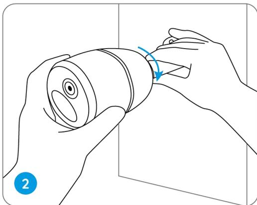
3. To get the best field of view, loosen the adjustment knob on security mount and turn the camera.
