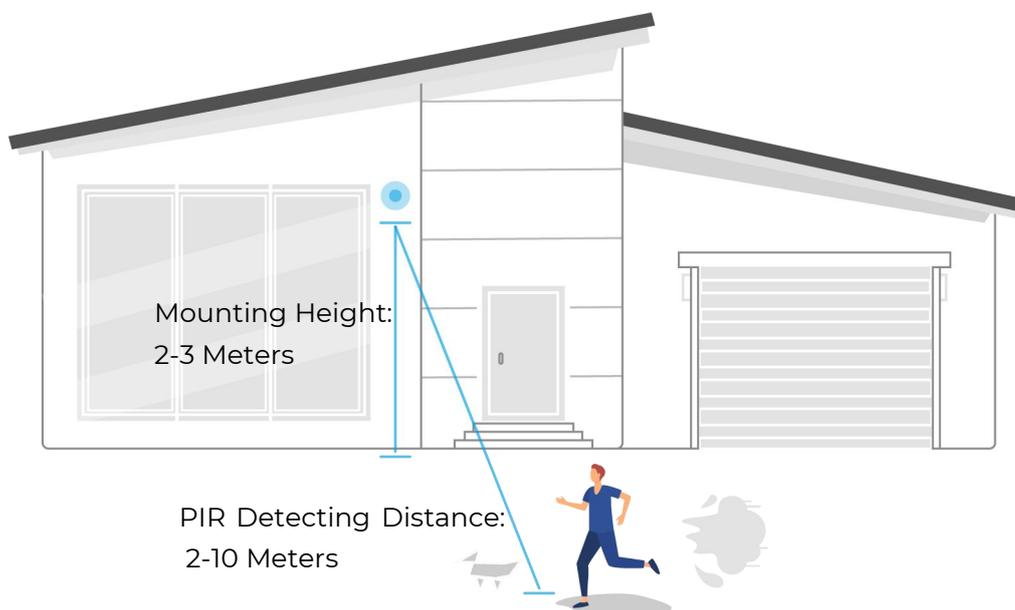
3. Adjust the installation height, it's suggested to mount a camera 2 to 3 meters from the ground. Mount the camera too low or too high both will cause it hard to detect alarm.
