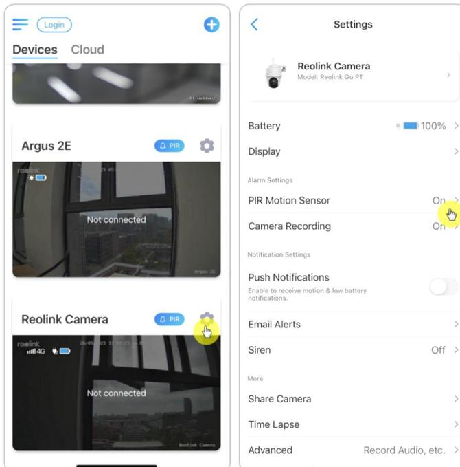
2. Tap to enable **PIR Motion Sensor**. Then tap **Schedule** to set up the schedule and decide when the PIR motion detection works.
