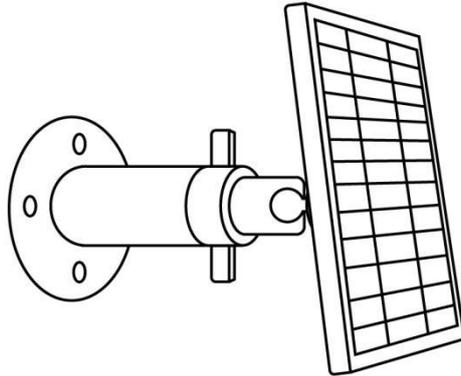
Step 4. Loosen the adjusting control on the bracket and adjust the angle of the Solar Panel to make it receive direct sunlight exposure, then tighten the adjusting control to fix the Solar Panel.
