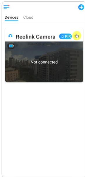
2. Tap on **Advanced** and then find **Record Audio**, tap to enable this option. Then the camera will record audio in video recordings.
