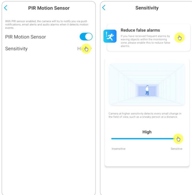
Drag the bar to adjust the sensitivity from low, mid to high or adjust the sensitivity from 1 to 100. For cameras with digital PIR sensors there's also an option to reduce false alarms.
