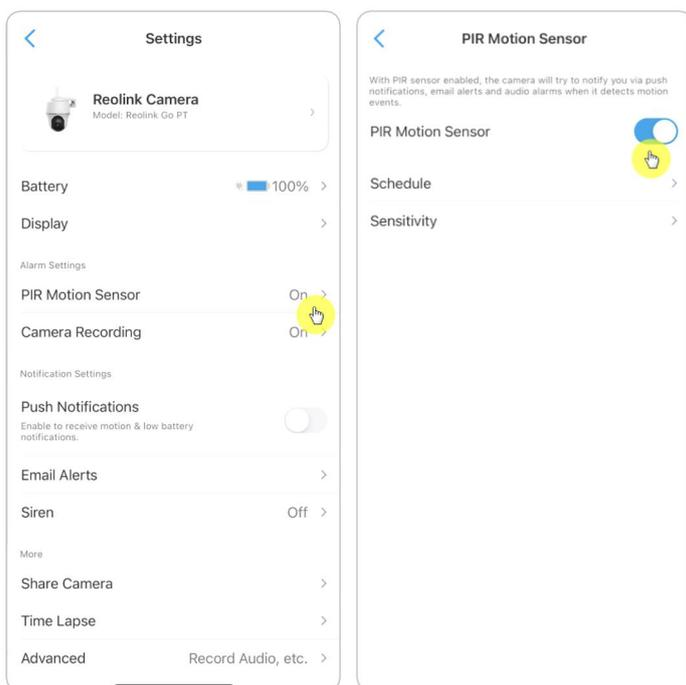
3. Tap **Sensitivity** to adjust the sensitivity of the PIR motion sensor.
