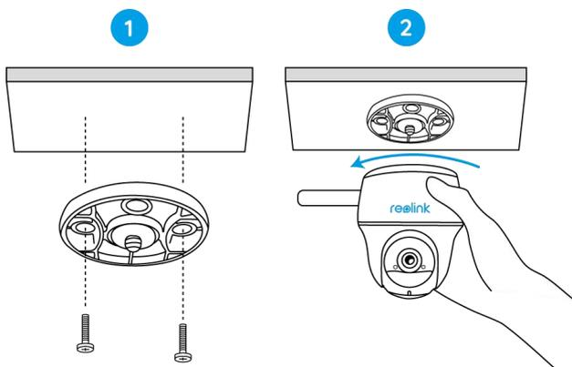
Install the bracket to the ceiling and attach the camera to it.
